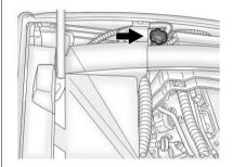
Remove the intercooler system pressure cap when the intercooler system hoses are no longer hot. Turn the pressure cap slowly counterclockwise about one-quarter of a turn. If you hear a hiss, wait for that to stop. This allows any pressure still left to be vented.
